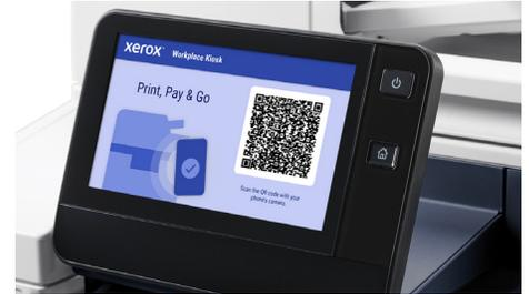
When users scan the QR code on the Kiosk welcome screen, their mobile device connects directly to the printer. To operate, they simply follow a series of screen prompts on their own device.
