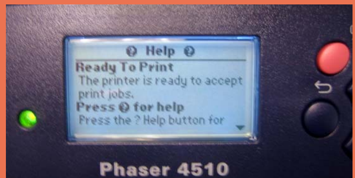
The printer's LCD panel provides a help screen that assists users with common questions and tasks.
