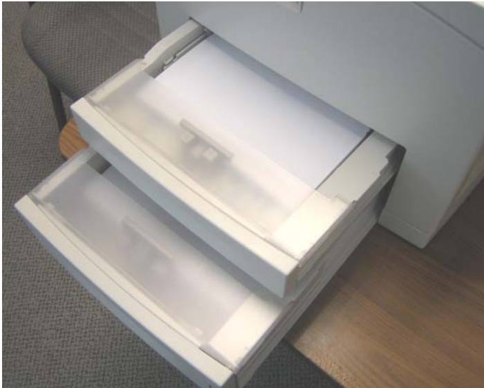
The Phaser 4510n's standard 150-sheet bypass tray and 550-sheet paper drawer.
