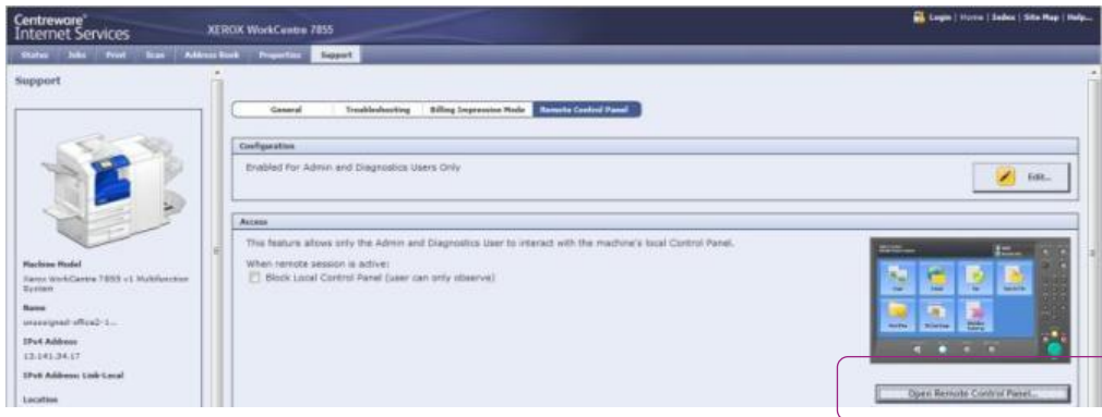
Screen shot showing Remote Control Panel tab and “Open Remote Control Panel” button in the Web UI.
