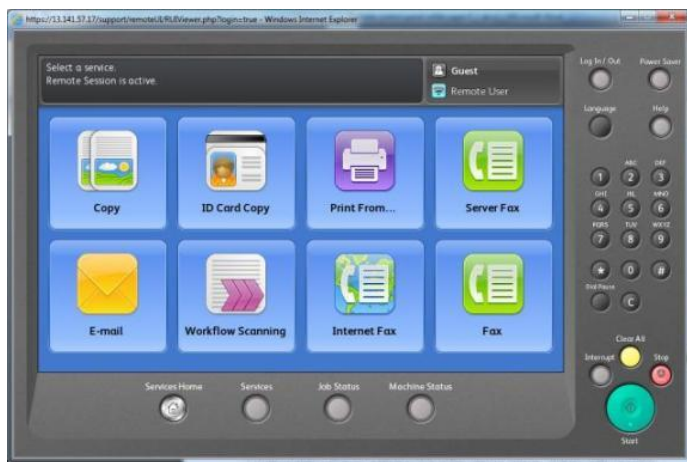
Screen shot of the ConnectKey Multifunction system user interface emulation displayed on a user PC. UI soft buttons and control panel hard buttons are fully operable using a local mouse and keyboard.
