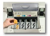
Unlike the HP Color LaserJet 4730mfp, which requires the user to remove and replace spent toner cartridges, the WorkCentre C2424's solid ink sticks are extremely easy to reload... new sticks need only be dropped into the unit's ink loader underneath the top cover and there are no empty cartridges that ever need to be removed. The HP's toner must be loaded from the side of the unit, adding to the already large floor area required for the device itself.
