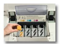
To change the toners on the Canon device, a user must go into the front panel menu, scroll to the Maintenance selection, and then scroll to the Change Cartridge selection. The user then must scroll to the correct toner color, select it for changing, and then wait for the cartridge cradle to rotate to the correct receptacle. Once the new cartridge is inserted, the device will then flash "PLEASE WAIT" a few minutes while the machine calibrates itself.
